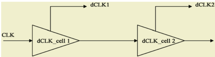
Fig. 2. dCLK\_cell chain for out-of-phase clock generation
