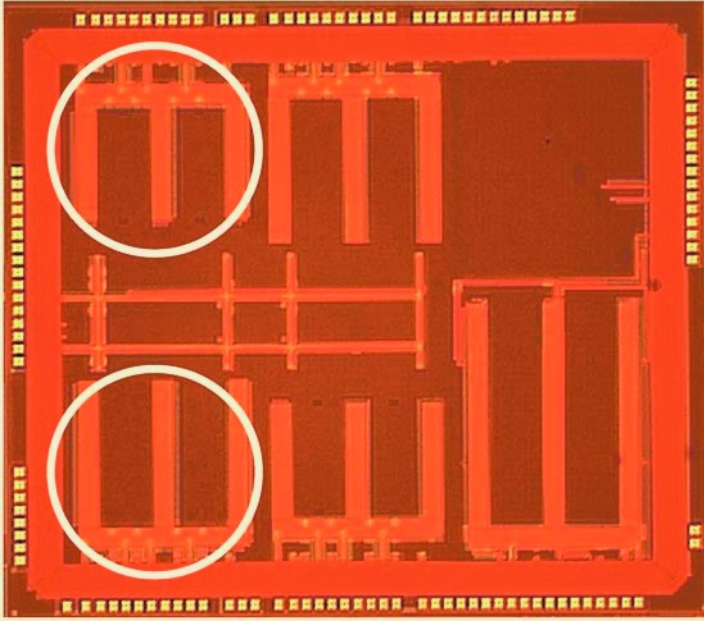
Fig. 4. Activity Monitor test chip. Upper circle: test circuit with normal flip-flops. Lower circle: test circuit with modified flip-flops including FFAMs.
